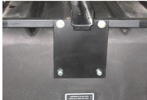
Now drill through one of the back corner holes of the frame and place a bolt in the hole to keep the frame in place while you drill out the remaining holes. From the inside of the body insert a 3/8" x 2" carriage bolt through the hole and secure the carriage bolt to the bottom of the frame using a 3/8" flat washer and 3/8" nylon locknut. **(Pliers may be required to hold the carriage bolt in place until it seats itself into the plastic)**
