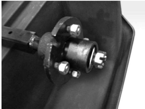
Place the hub assembly, spindle washer, and spindle nut on the end of the axel as pictured. Tighten the spindle nut until the hub bearing and washer are tight against the back of the axel, the rotation of the hub should be difficult. Loosen off the nut 1/4 – 1/2 a turn so that the hole in the axel is centered between two of the notches in the spindle nut.
