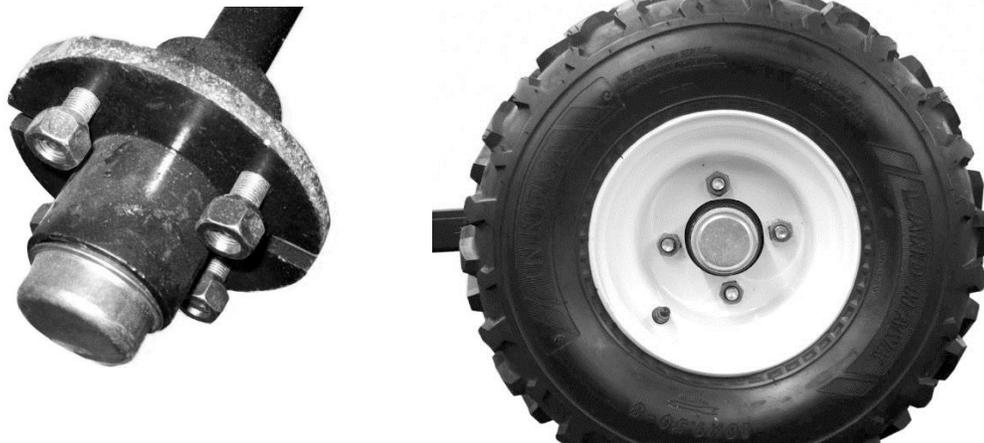
Place dust cap on hub. Using a rubber mallet, tap into place. Finally remove the hub nuts and place tire and rim onto the hub so the valve stem is facing out and tighten tire onto hub. Repeat for the other side.
